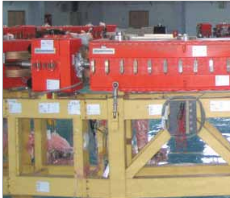
Parts of the BESSY 1 0.8 GeV booster synchrotron as they arrived from Germany to be assembled at the SESAME facility
